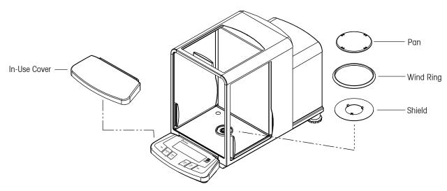
Installation of Balance Components
