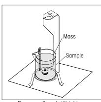
Buoyancy Sample Weighing
