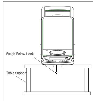
Balance With Weigh Below Hook Installed
