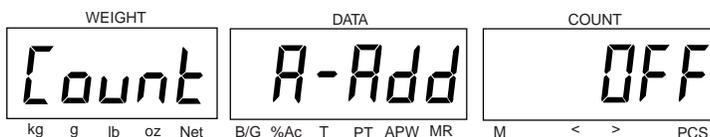
Print Clear - When Print clear is set to ON, the Scale prints the accumulated count memory and then clears the accumulated memory when the **PRINT Units** button is pressed. Select ON or OFF.
