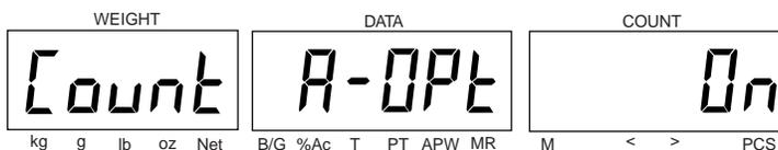
Memory Change - A 10d weight change is required before the accumulated memory can be changed by pressing **M+** or **M-**. Select ON or OFF.
