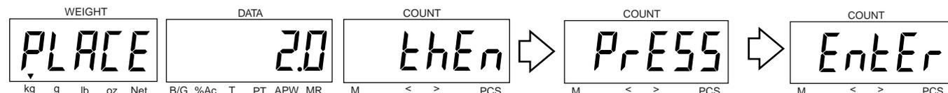
Place the indicated calibration mass on the pan, then press the **Enter** button. The sample illustration indicates a 6kg Scale using a 2kg mass.
