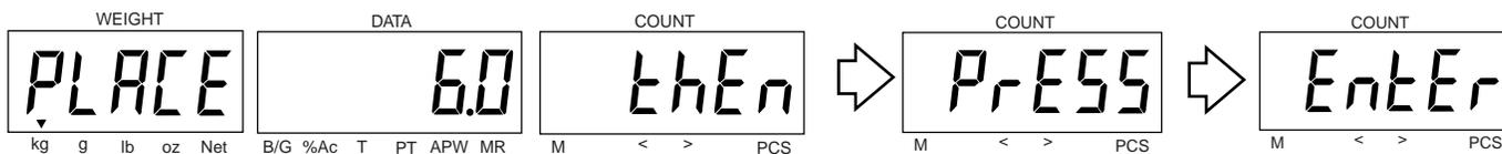
Place the indicated calibration mass on the pan. Press the **Enter** button. The sample illustration indicates a 6kg Scale using a 6kg mass.
