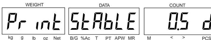
Print Header - Allows printing of preset header that includes OHAUS, Model No. and unit serial number. Select ON or OFF.
