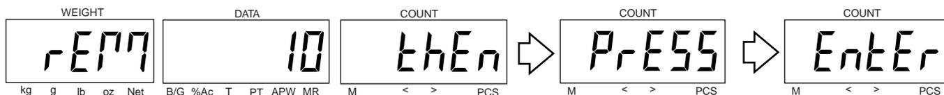
Remove 10 pieces as instructed, or use the keypad to change the number of pieces to be removed, then press **Enter** button.
